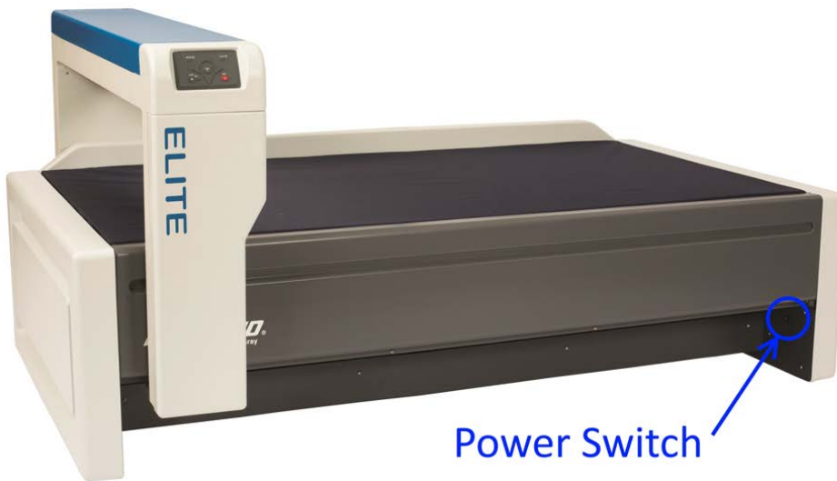
Figure 4-16: Power Switch location
