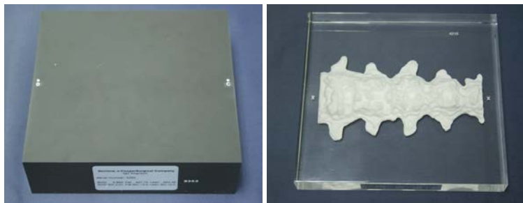
Figure 4-5: Black (Body Composition) and Clear (Bone Only) QC Phantoms
