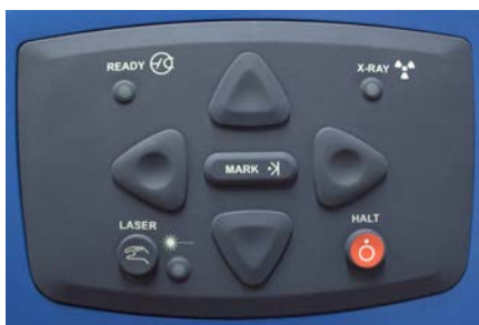
Figure 2-3: Scanner Arm Touch Pad
