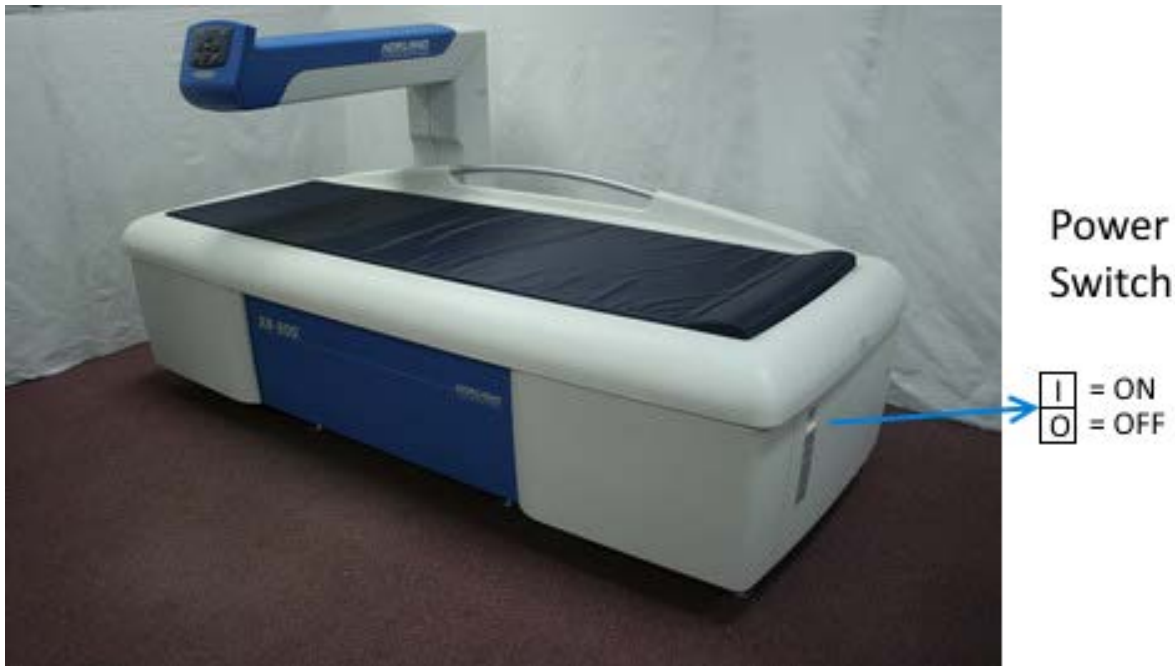
Figure 1-1: Power Switch location
