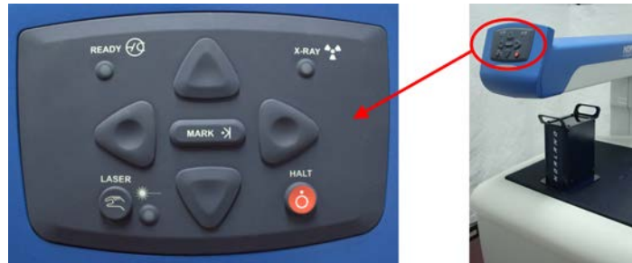
Figure 1-2: Scanner Touch Pad
