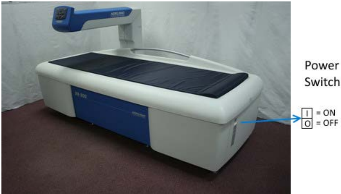
Figure 1-1: Power Switch location
